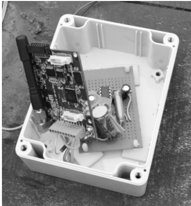
Figure 4a. Transmission node and boost converter
